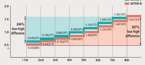
The table at left shows the relative gear ratio for the Inter-7 and Inter-8 gear hubs when used with a 20T sprocket. The numbers in parenthesis show the sprocket size that each gear ratio corresponds to in a derailleur system.
